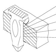
Nominal hole diameter Ø1,0 mm Diameter of the hole prior to plating Ø1,15±0,025 mm Cu plating 0,025-0,075 mm SnPb plating 0,005-0,015 mm Diameter of the finished hole Ø0,94-1,09 mm
